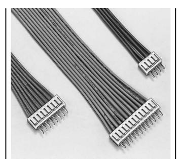
Measuring 2.0mm (.079") in pitch, 6.0mm (.236") in mounting height, and 3.25mm (.128") in thickness, this board-in connector meets the needs for high-density mounting on printed circuit boards efficiently and economically.
