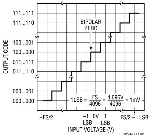
Figure 10c. LTC1277 Bipolar Transfer Characteristics (Offset Binary)
