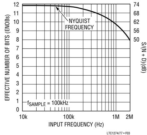
Figure 3. ENOBs and S/(N + D) vs Input Frequency
