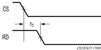
$\overline{\text{CS}}$  to  $\overline{\text{CONVST}}$  Setup Timing
