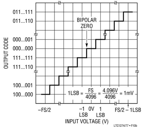
Figure 10b. LTC1274 Bipolar Transfer Characteristics (2's Complement)
