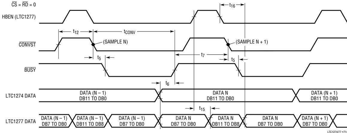
Figure 14. Mode 1b.  $\overline{CONVST}$  Starts a Conversion. Data Outputs Always Enabled
