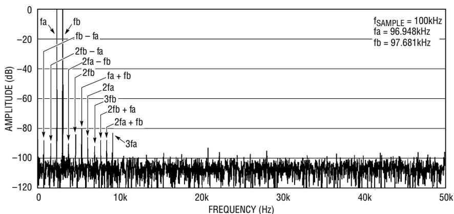
Figure 5. Intermodulation Distortion
