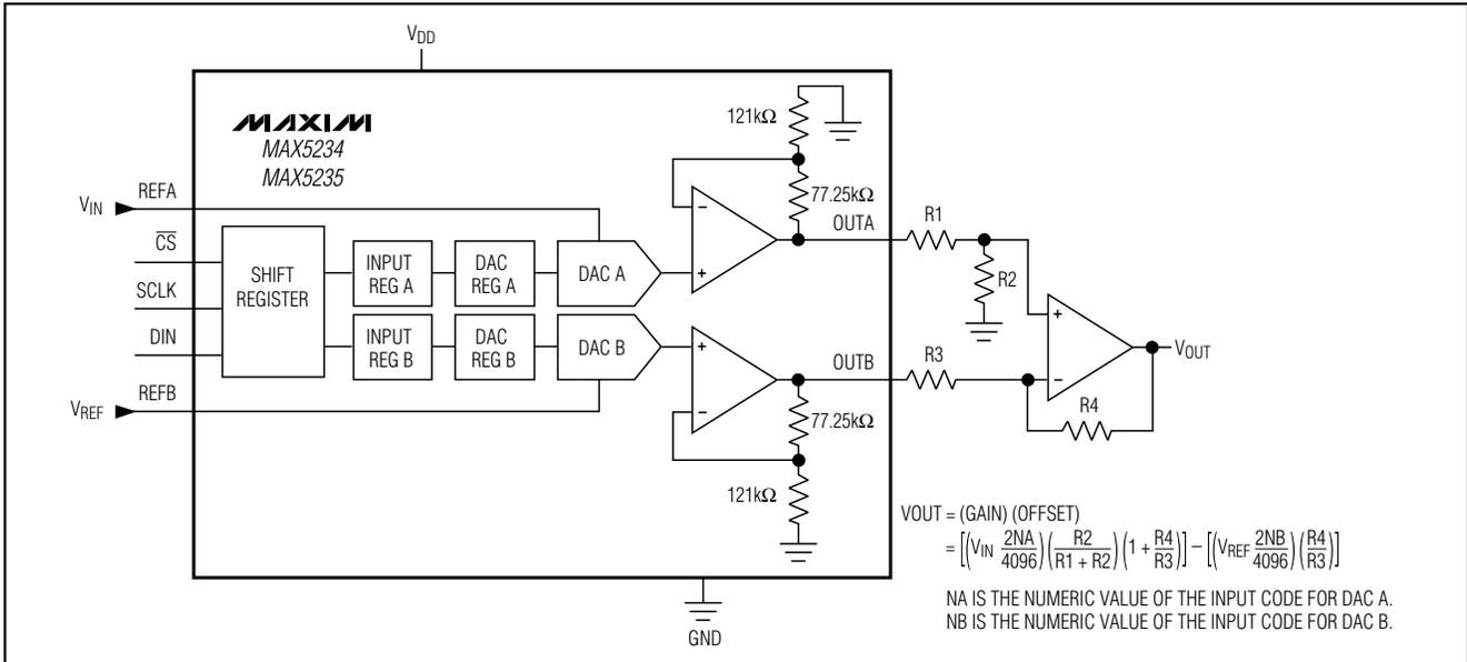
Figure 11. Digital Control of Gain and Offset
