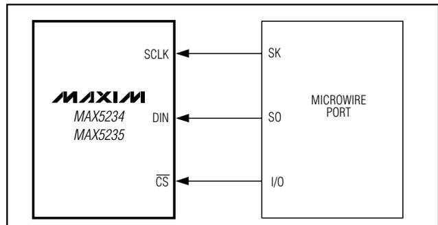
Figure 5. Connections for MICROWIRE
