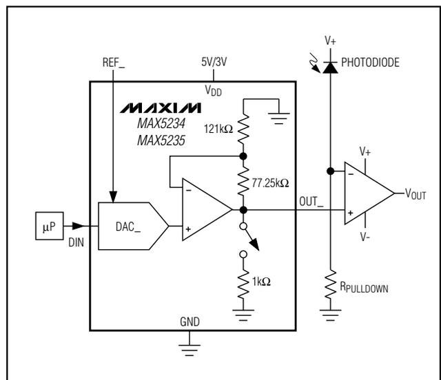
Figure 10. Digital Calibration
