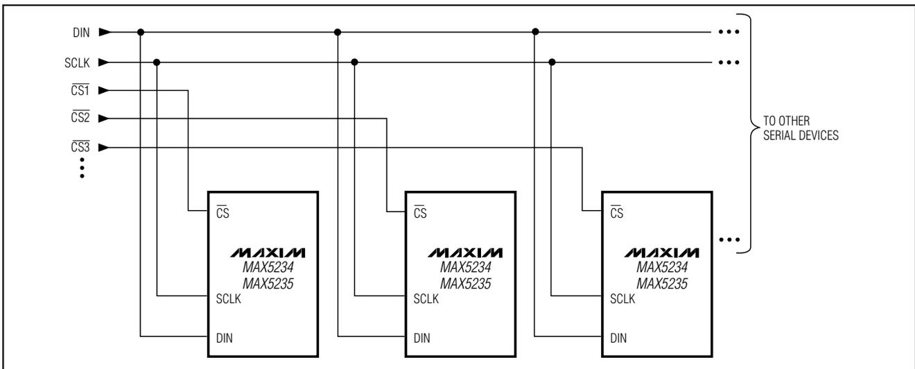
Figure 12. Multiple MAX5234/MAX5235 Sharing a Common DIN Line
