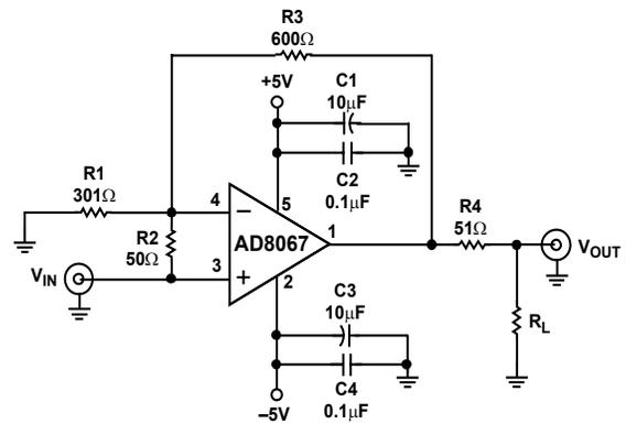
Figure 54. Gain of Less than 2 Schematic
