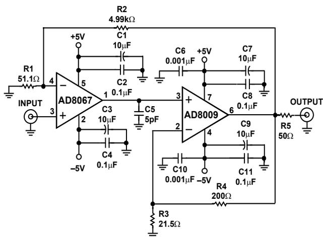
Figure 57. AD8067/AD8009 Composite Amplifier  $A_v = 100$ , GBWP = 6.1 GHz
