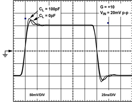
Figure 19. Small Signal Transient Response  $\pm 5$  V Supply
