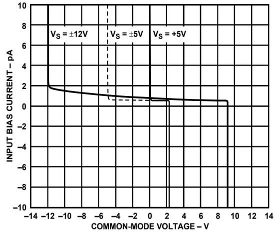
Figure 25. Input Bias Current vs. Common-Mode Voltage
