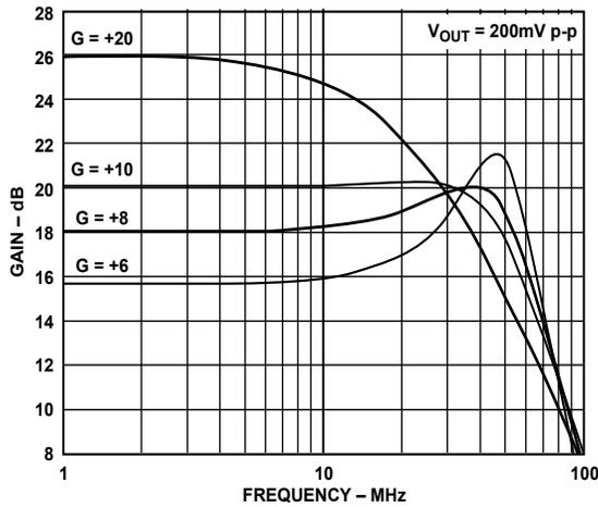
Figure 4. Small Signal Frequency Response for Various Gains
