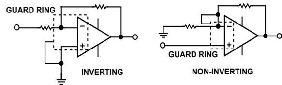
Figure 47. Guard-Ring Configurations
