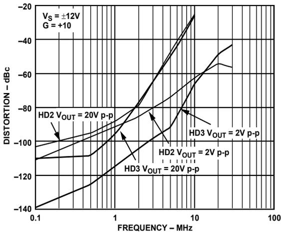
Figure 12. Distortion vs. Frequency for Various Amplitudes
