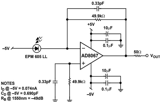
Figure 51. Photodiode Preamplifier
