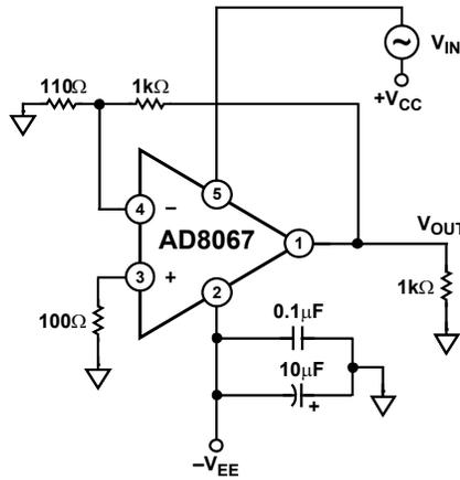
Figure 38. Positive PSRR Test Circuit
