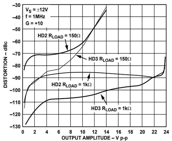
Figure 15. Distortion vs. Output Amplitude for Various Loads
