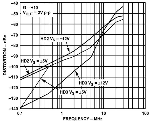
Figure 14. Distortion vs. Frequency for Various Supplies
