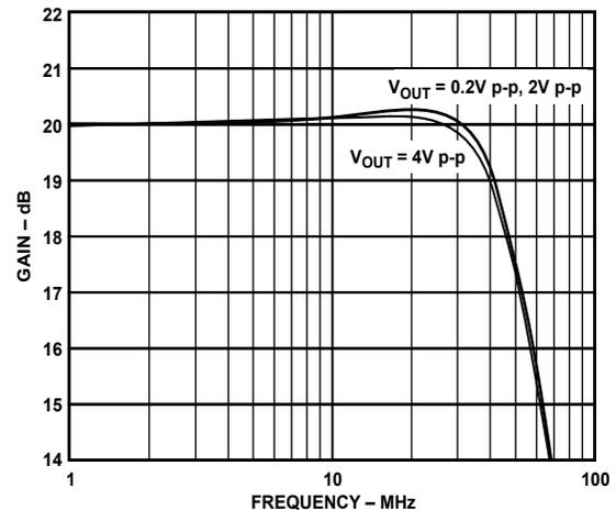
Figure 9. Frequency Response for Various Output Amplitudes
