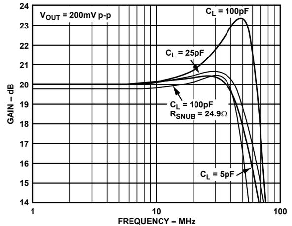
Figure 8. Small Signal Frequency Response for Various  $C_{LOAD}$
