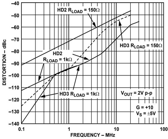
Figure 11. Distortion vs. Frequency for Various Loads
