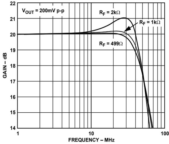
Figure 10. Small Signal Frequency Response for Various  $R_f$
