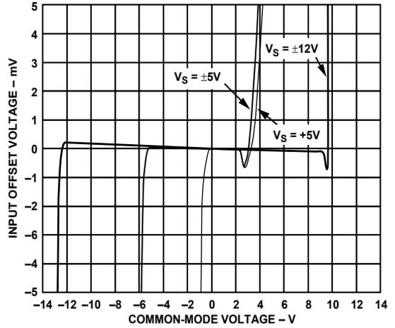
Figure 26. Input Offset Voltage vs. Common-Mode Voltage
