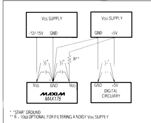
Figure 14. Power-Supply Grounding
