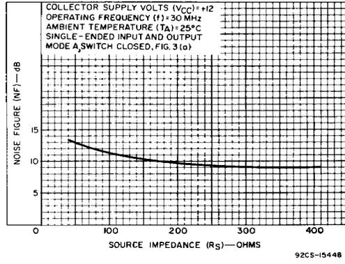
Fig.8 - Noise Figure (NF) vs Source Impedance
