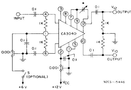
\* VARIABLE CAPACITANCE (0.5-10 μF) ADJUSTMENT FOR EQUAL 3dB BANDWIDTH AT AMPLIFIER OUTPUTS, TERMINALS 10 AND 12.
