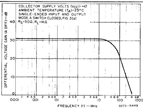
Fig.4 - Differential Voltage Gain vs Frequency
