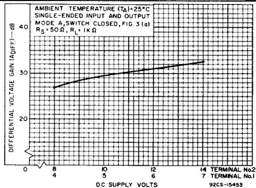
Fig.5 - Differential Voltage Gain vs DC Supply Voltages
