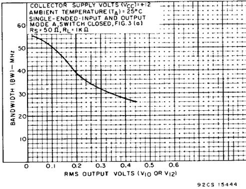
Fig.7 - 3dB Bandwidth vs Single-Ended Output Voltage
