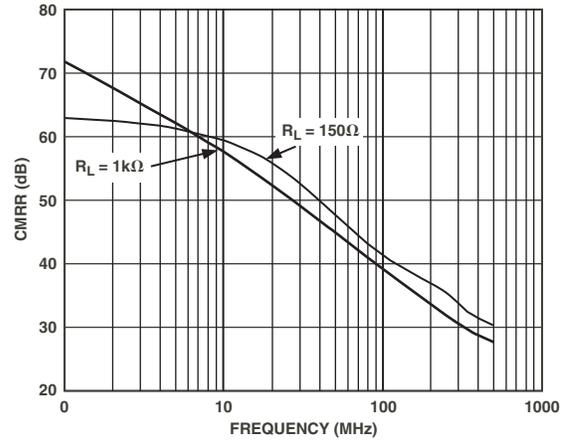
TPC 24. Common-Mode Rejection Ratio, CMRR ( $R_S = 100 \Omega$ )
