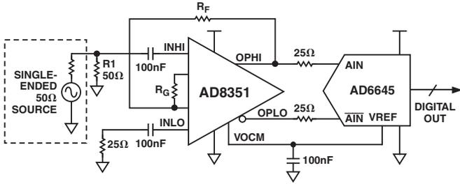
Figure 8. ADC Driving Application Using Single-Ended Input
