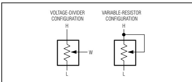
Figure 1. Voltage-Divider/Variable-Resistor Configurations
