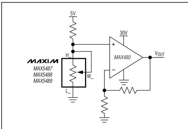
Figure 5. Positive LCD-Bias Control Using a Variable Resistor
