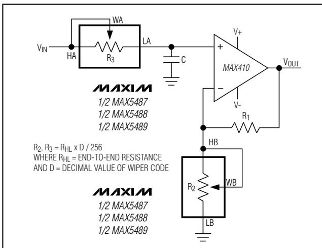
Figure 6. Programmable Filter
