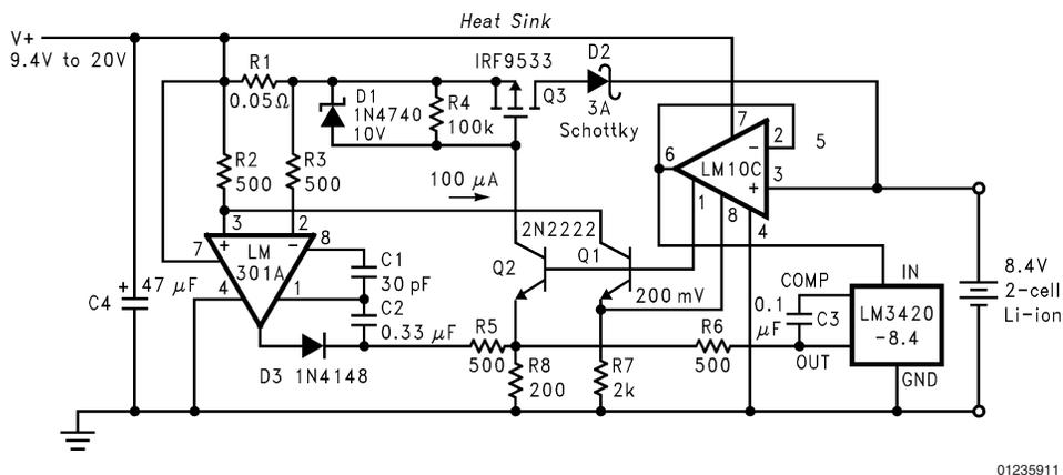
FIGURE 6. Low Drop-Out Constant Current/Constant Voltage 2-Cell Charger
