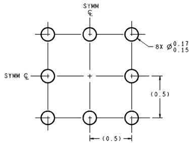
DIMENSIONS ARE IN MILLIMETERS
