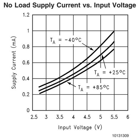
**Typical Performance Characteristics** Unless otherwise specified,  $T_A = 25^\circ\text{C}$ ,  $V_{\text{OUT}} = -2.5\text{V}$ . (Continued)
