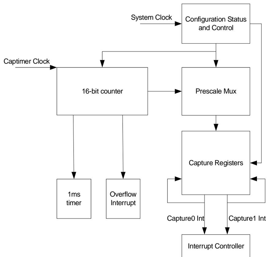
**Figure 11-3. Timer Capture Block Diagram**
