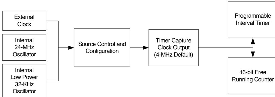
**Figure 17-2. Time Capture Block Diagram**
