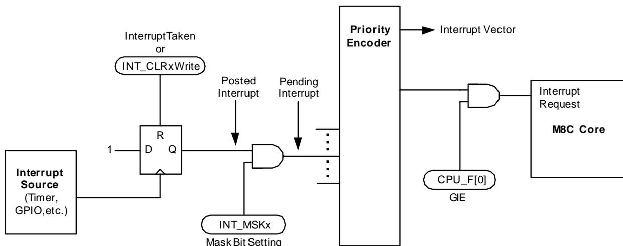
**Figure 18-1. Interrupt Controller Block Diagram**
