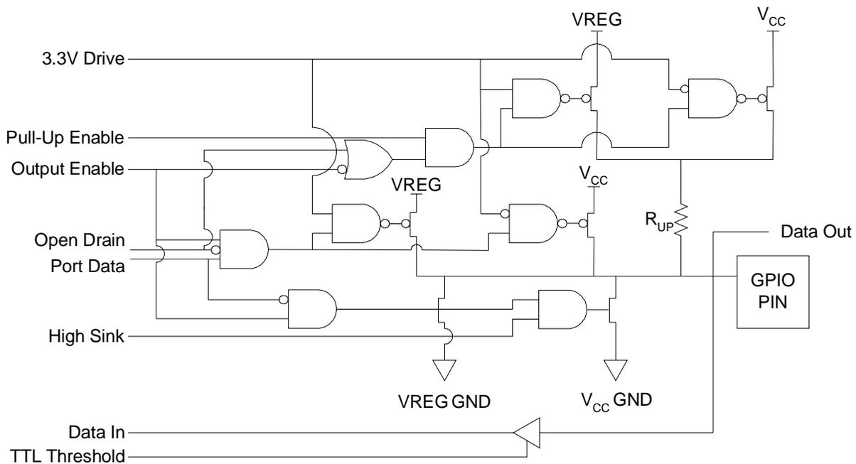
**Figure 15-1. GPIO Block Diagram**
