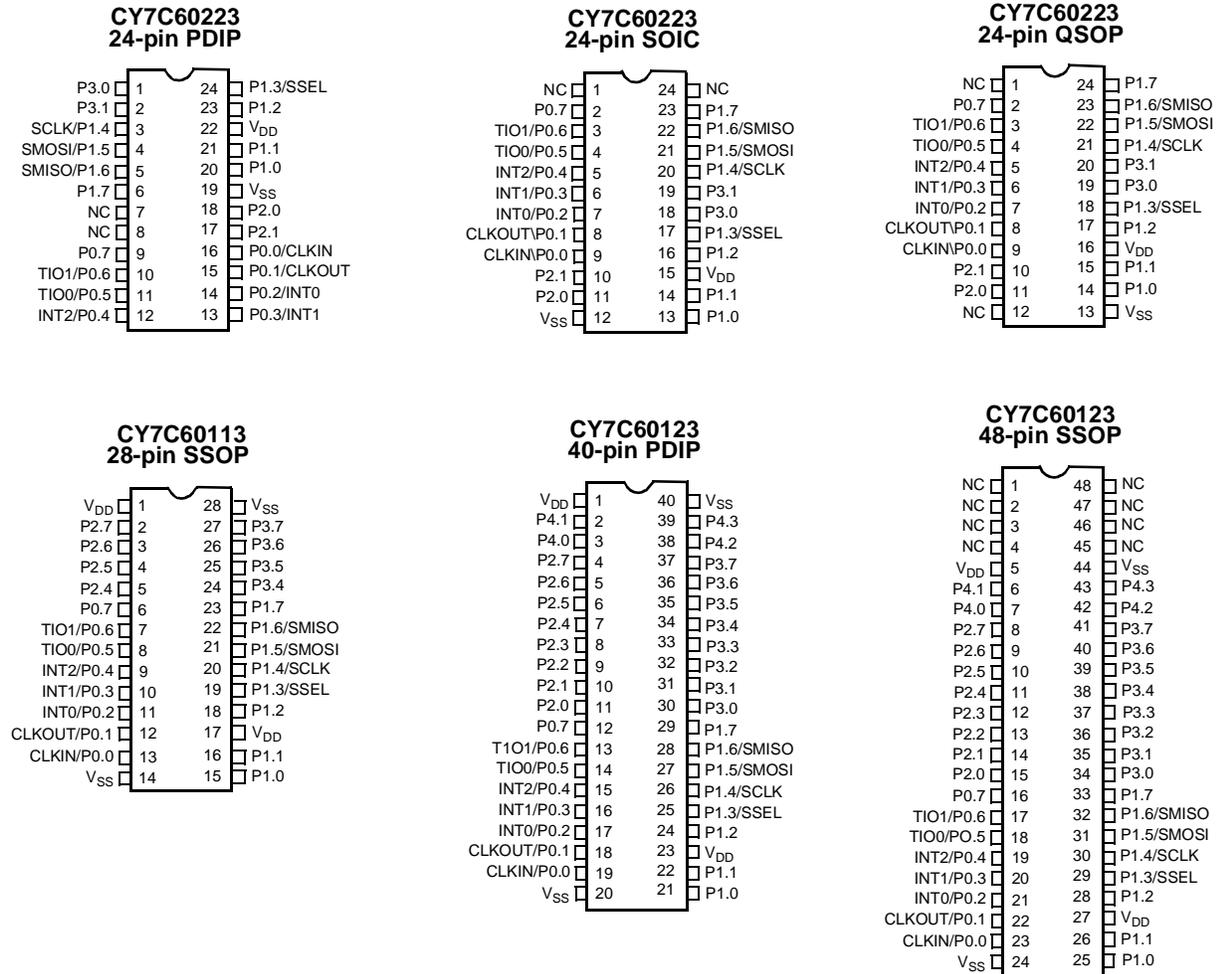
**Figure 5-1. Package Configurations**
