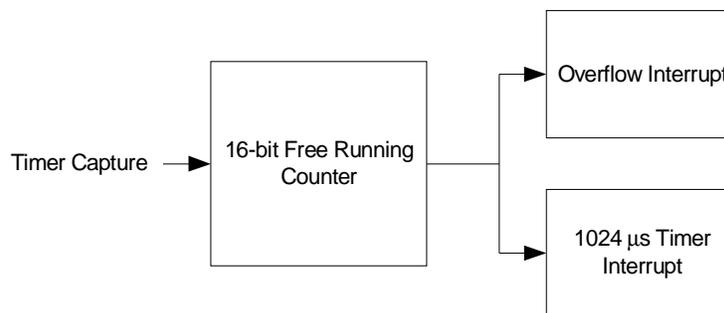
**Figure 17-1. 16-bit Free Running Counter Block Diagram**
