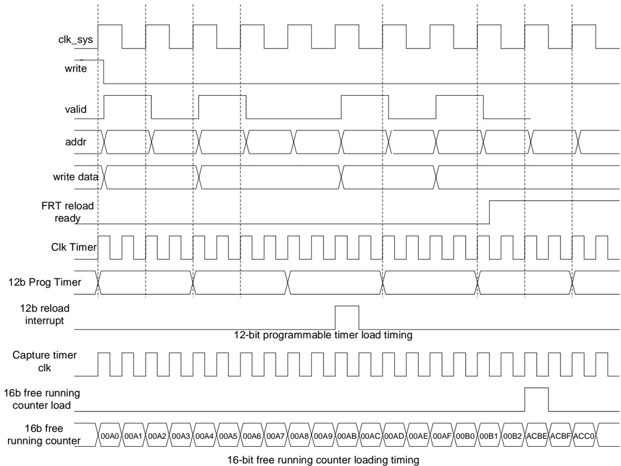
**Figure 17-4. 16-bit Free Running Counter Loading Timing Diagram**
