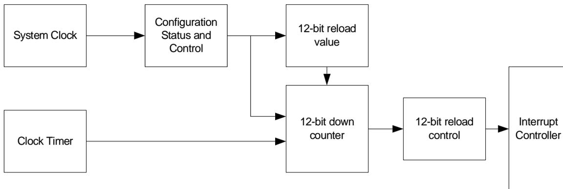
**Figure 11-2. Programmable Interval Timer Block Diagram**
