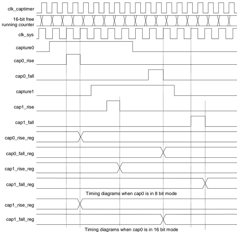
**Figure 17-3. Timer Functional Timing Diagram**
