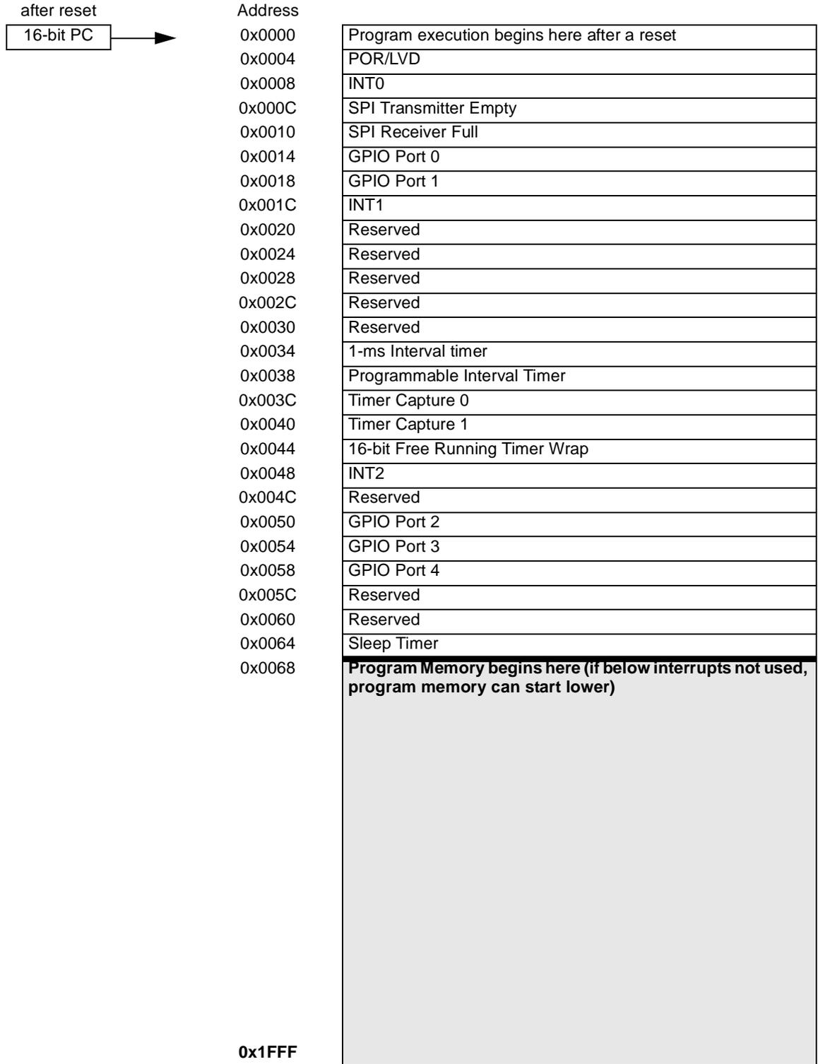
Figure 10-1. Program Memory Space with Interrupt Vector Table
