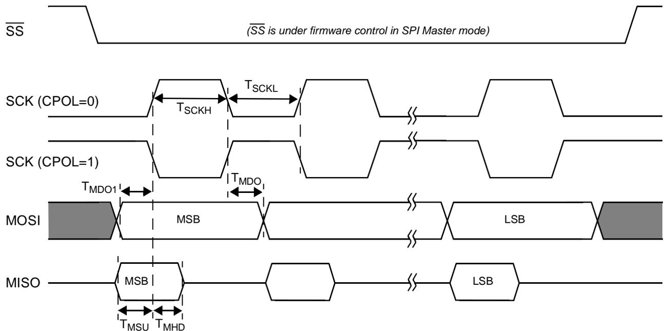
Figure 21-4. SPI Master Timing, CPHA = 0
