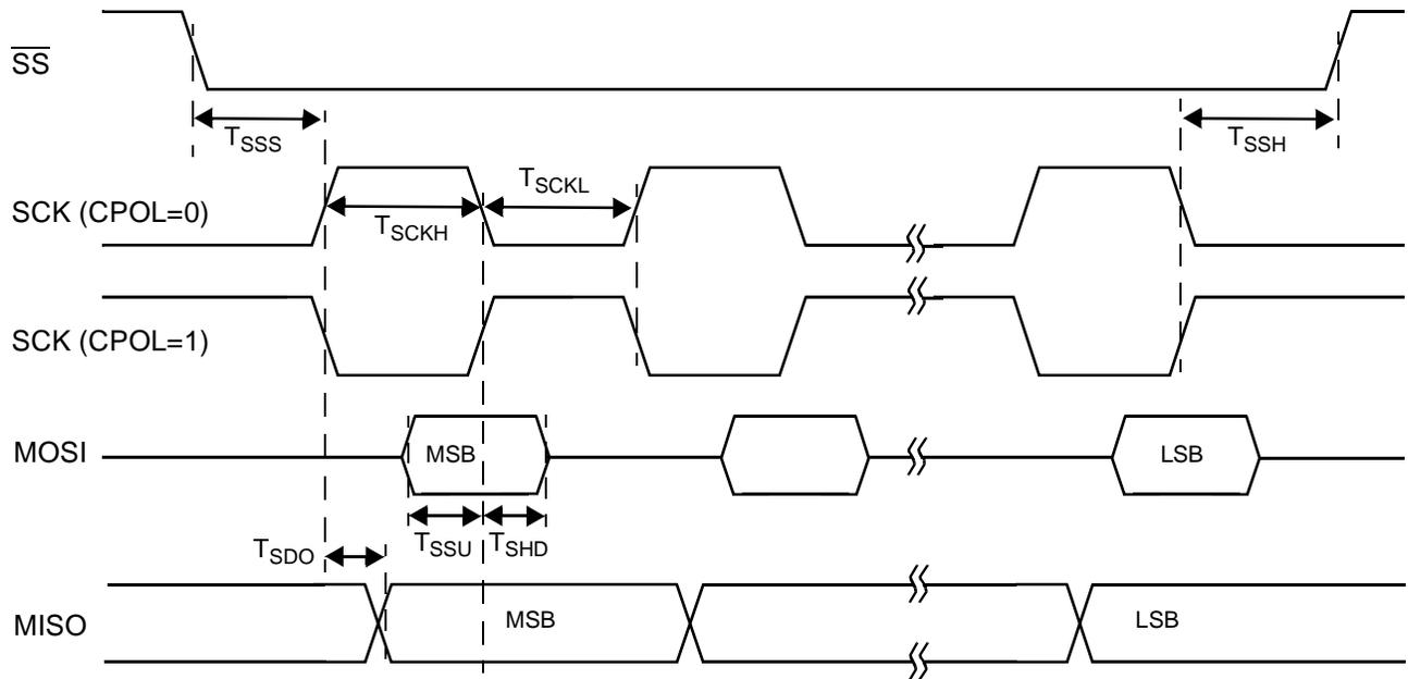
Figure 21-3. SPI Slave Timing, CPHA = 1
