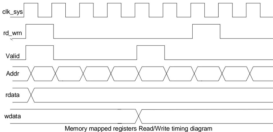
**Figure 17-5. Memory Mapped Registers Read/Write Timing Diagram**
