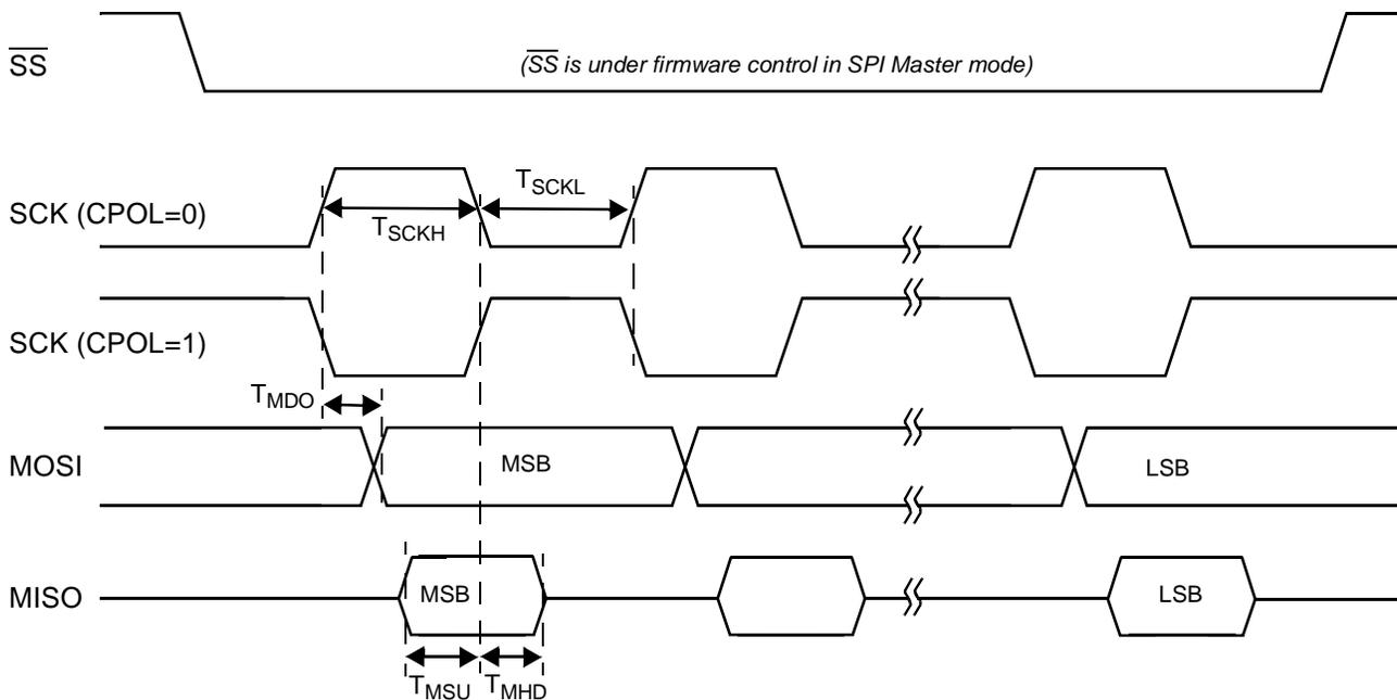
**Figure 21-2. SPI Master Timing, CPHA = 1**
