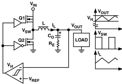
Figure 1. Conventional Hysteretic Regulator and Its Characteristic Waveforms
