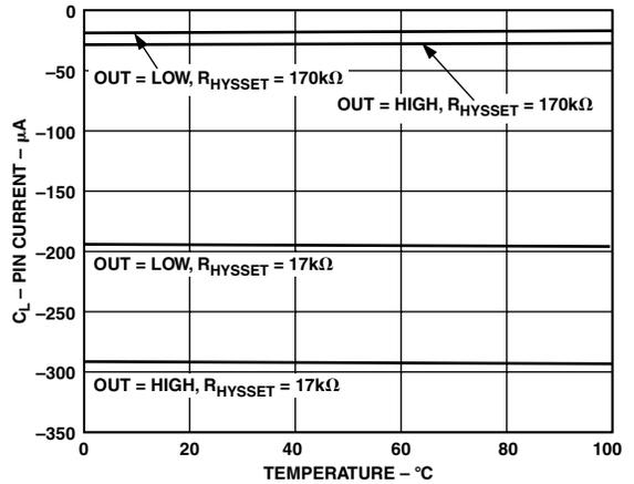
TPC 5. Current Limit Programming Current vs. Temperature
