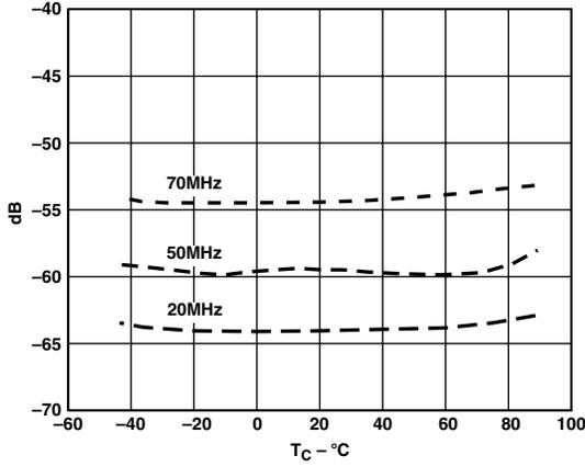
Figure 21. 2nd Harmonic vs. Temperature:  $f_S = 200$  MSPS
