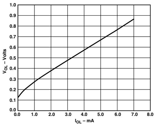
Figure 29. Output Voltage LOW vs. Output Current
