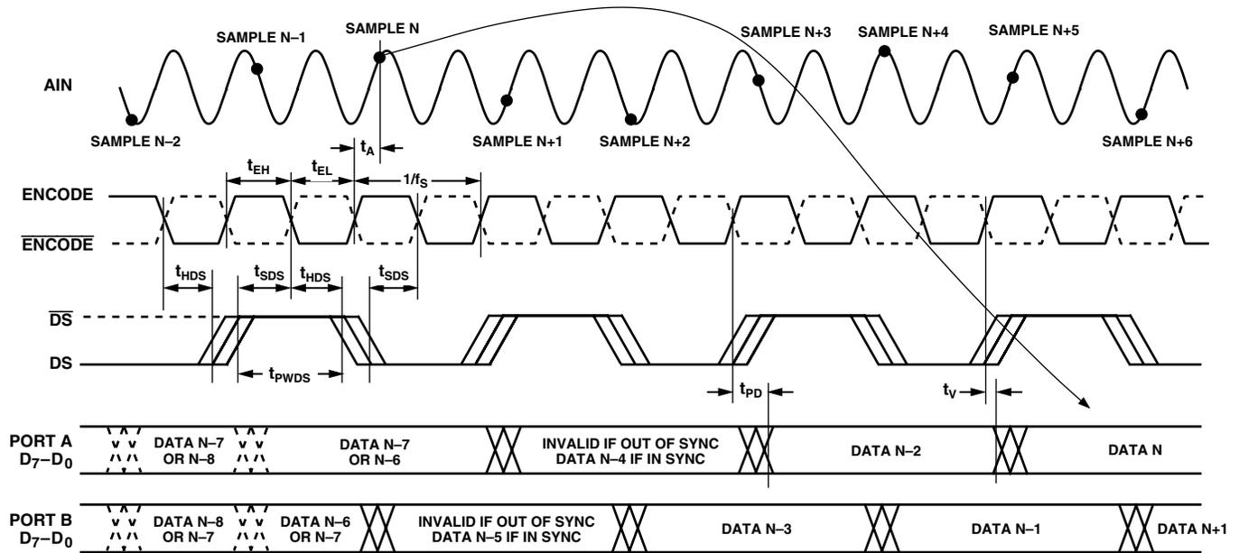
Figure 2b. Timing—Dual Channel Mode (Continuous Data Sync)
