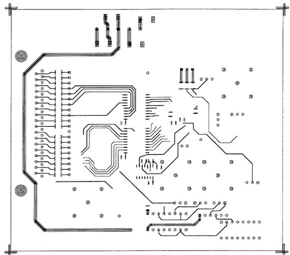
Figure 42. Conductors—Bottom View
