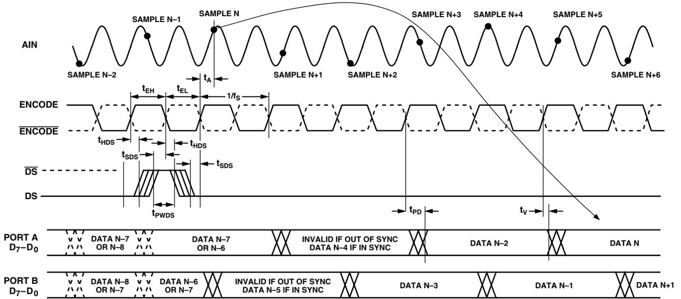
Figure 2a. Timing—Dual Channel Mode (One-Shot Data Sync)
