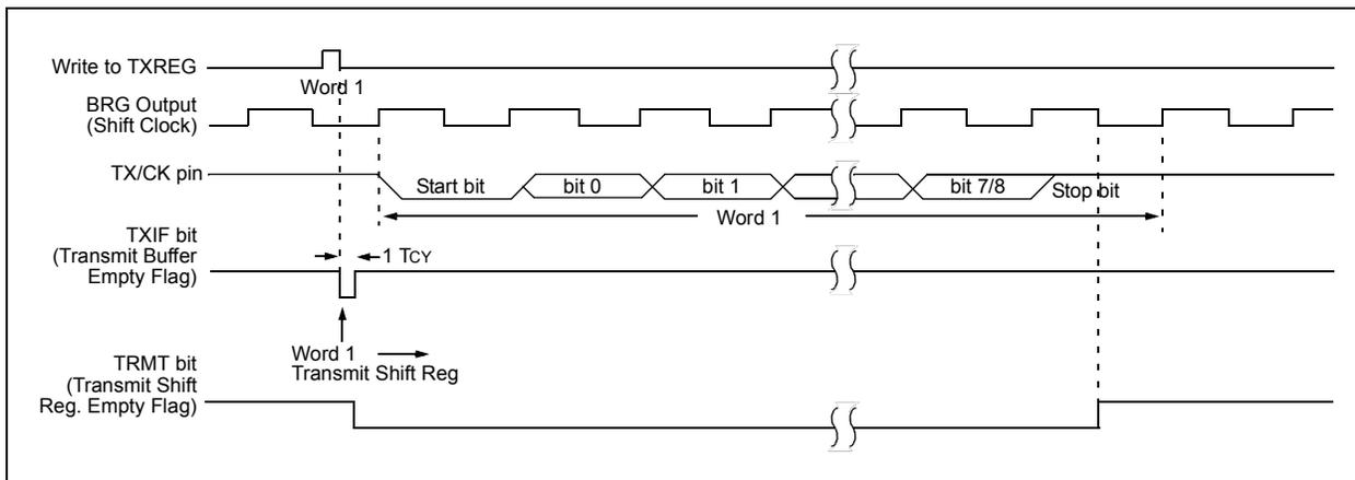
**FIGURE 9-4: ASYNCHRONOUS TRANSMISSION (BACK-TO-BACK)**
