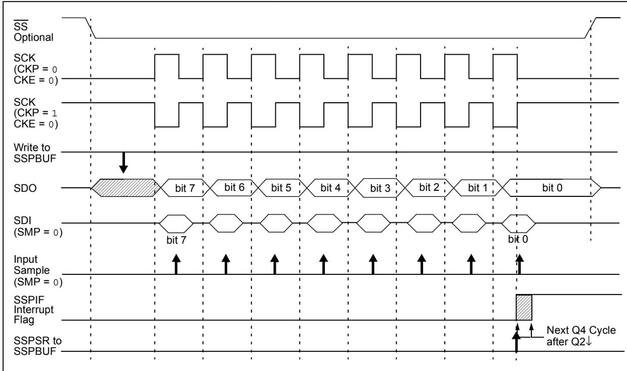
**FIGURE 14-6: SPI MODE WAVEFORM (SLAVE MODE WITH CKE = 1)**
