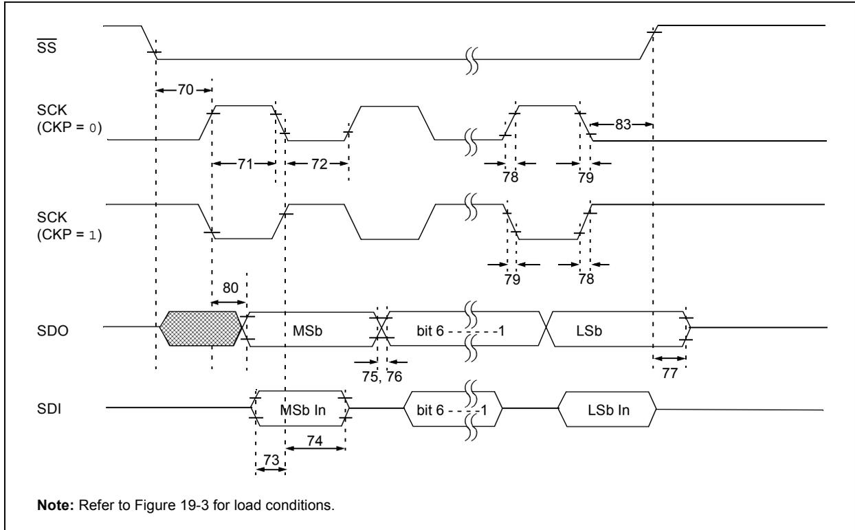
**FIGURE 19-17: SPI SLAVE MODE TIMING (CKE = 1)**
