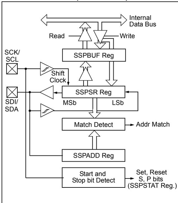
The SSP module has five registers for the I<sup>2</sup>C operation, which are listed below.
