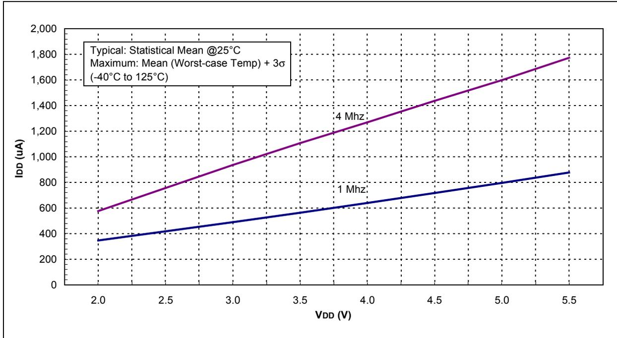
**FIGURE 20-9: I<sub>DD</sub> vs. V<sub>DD</sub> OVER F<sub>osc</sub> (LFINTOSC MODE, 31 kHz)**
