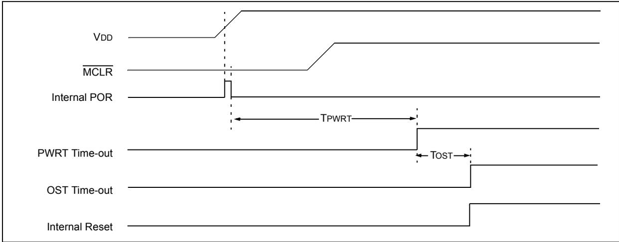
**FIGURE 16-5: TIME-OUT SEQUENCE ON POWER-UP (DELAYED  $\overline{\text{MCLR}}$ ): CASE 2**
