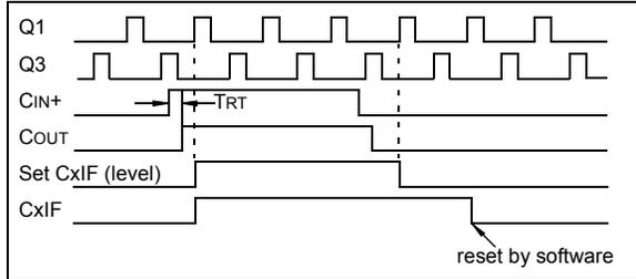
**FIGURE 8-7: COMPARATOR INTERRUPT TIMING WITH CMCON0 READ**
