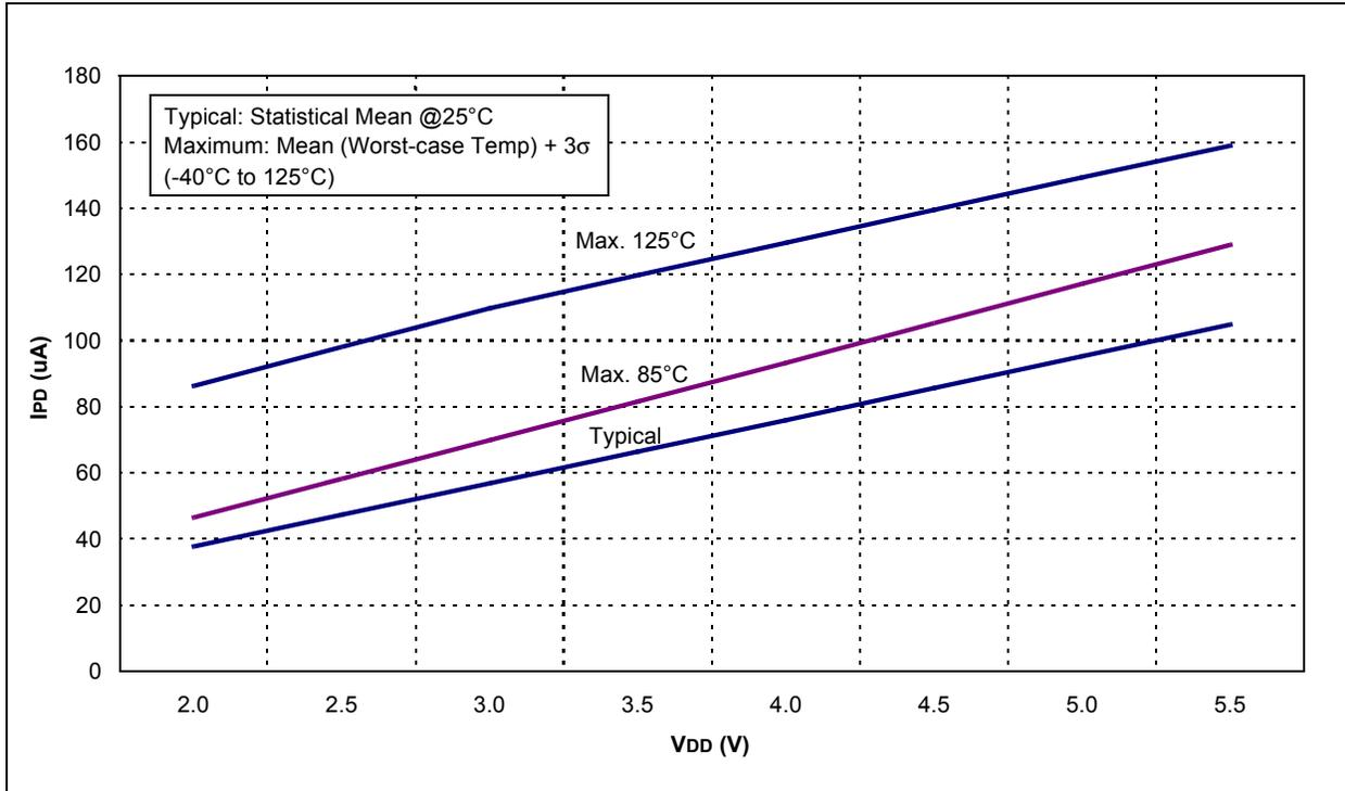
FIGURE 20-23: LVD IPD vs. VDD OVER TEMPERATURE
