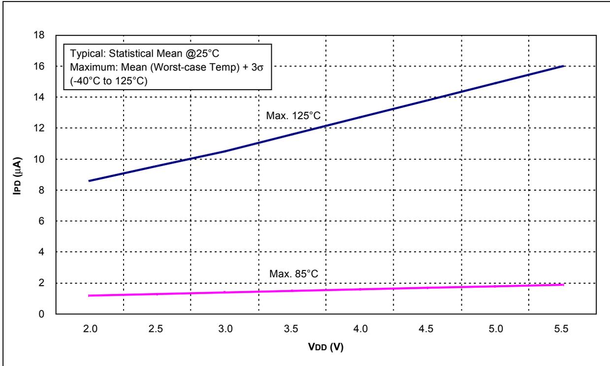
FIGURE 20-15: COMPARATOR IPD vs. VDD (BOTH COMPARATORS ENABLED)
