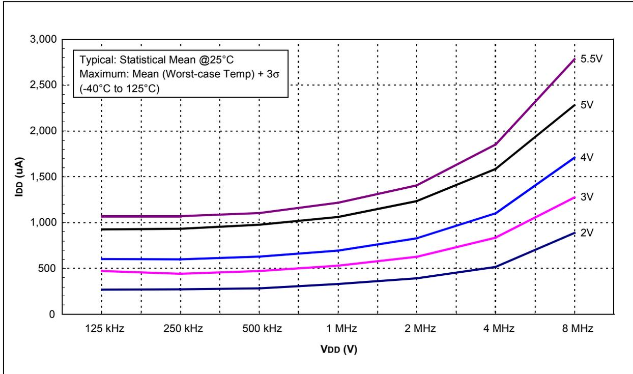
FIGURE 20-13: TYPICAL  $I_{PD}$  vs.  $V_{DD}$  (SLEEP MODE, ALL PERIPHERALS DISABLED)
