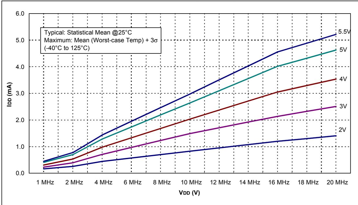
**FIGURE 20-3: TYPICAL I<sub>DD</sub> vs. F<sub>osc</sub> OVER V<sub>DD</sub> (HS MODE)**
