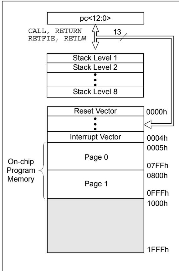
**FIGURE 2-2: PROGRAM MEMORY MAP AND STACK FOR THE PIC16F916/917/PIC16F946**
