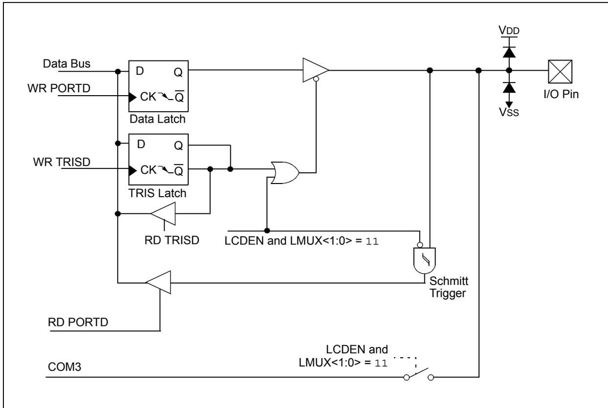
FIGURE 3-23: BLOCK DIAGRAM OF RD1
