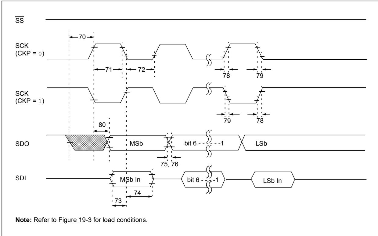
**FIGURE 19-15: SPI MASTER MODE TIMING (CKE = 1, SMP = 1)**
