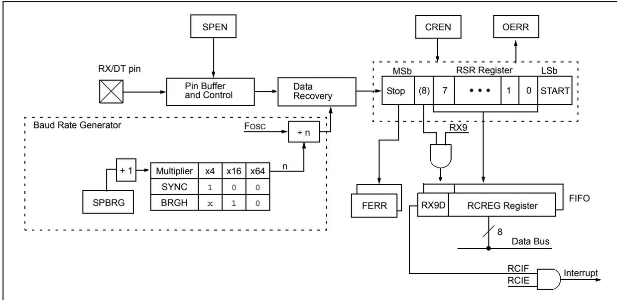
The operation of the AUSART module is controlled through two registers:
