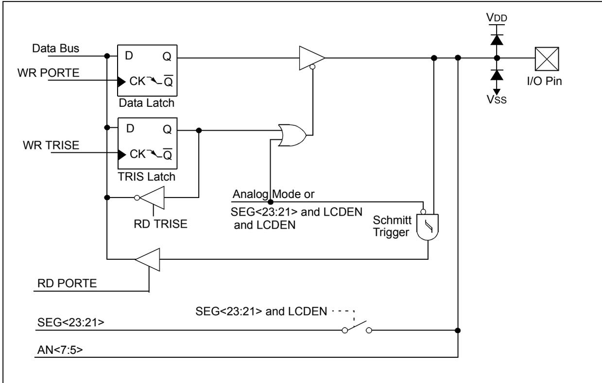
FIGURE 3-27: BLOCK DIAGRAM OF RE3
