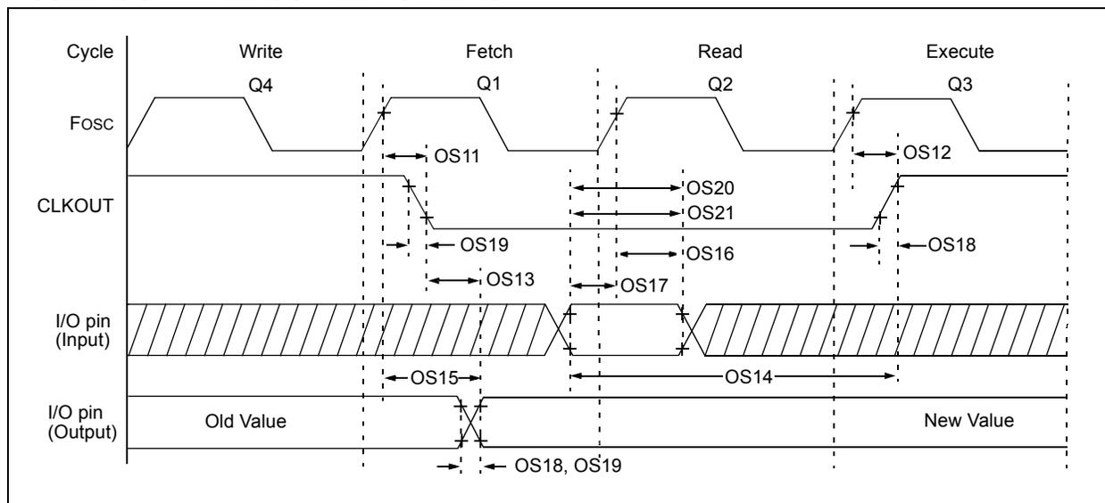
**TABLE 19-3: CLKOUT AND I/O TIMING PARAMETERS**
