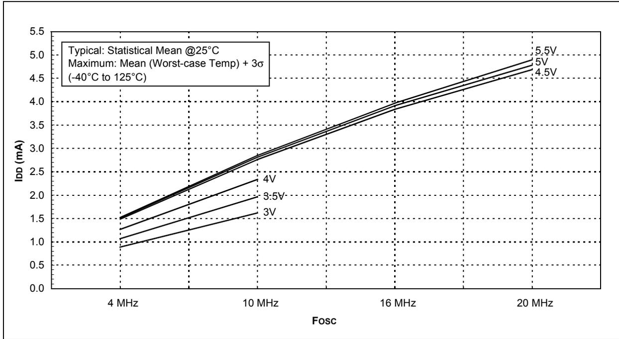
**FIGURE 20-5: TYPICAL I<sub>DD</sub> vs. V<sub>DD</sub> OVER F<sub>osc</sub> (XT MODE)**
