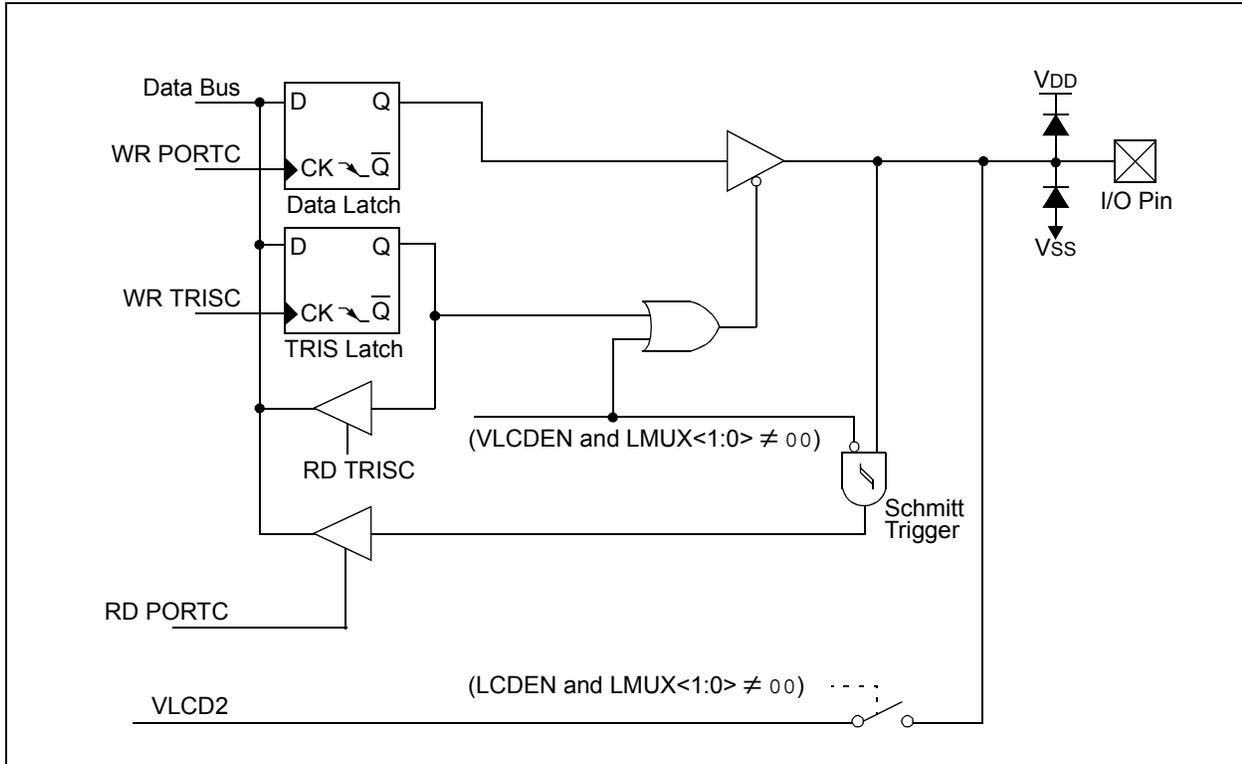
FIGURE 3-16: BLOCK DIAGRAM OF RC2
