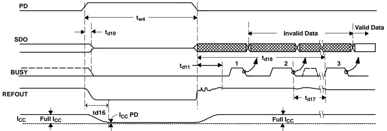
Figure 53. Device Full Power Down/Resume (Internal Reference Used)
