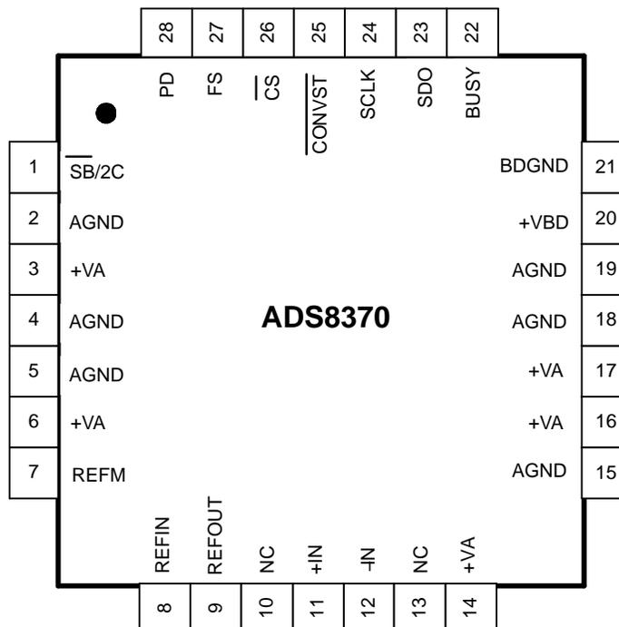
Note: The package thermal pad must be soldered to the printed circuit board for thermal and mechanical performance.
