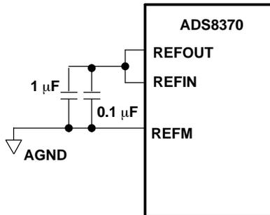
**Figure 48. ADS8370 Using Internal Reference**
