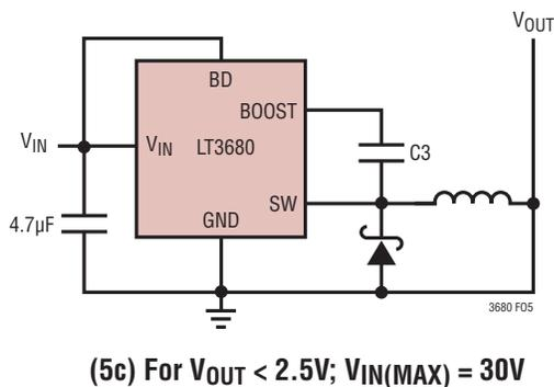
Figure 5. Three Circuits For Generating The Boost Voltage
