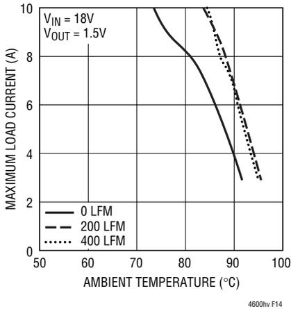
Figure 14. BGA Heatsink
