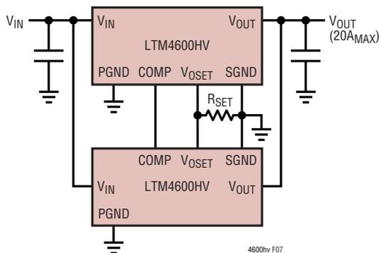
Figure 7. Parallel Two  $\mu$ Modules with Load Sharing
