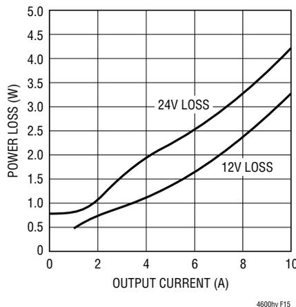
Figure 15. 3.3V Power Loss Curves vs Load Current
