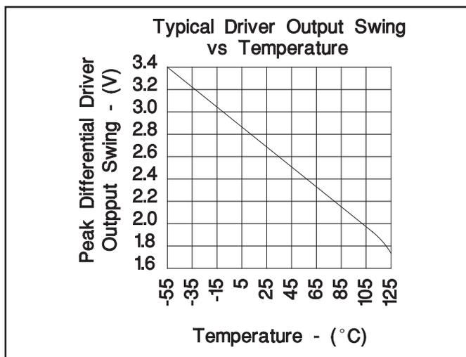
Figure 3. Typical Driver Output Swing vs Temperature
