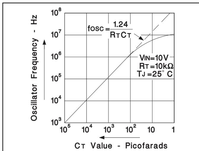
Figure 2. Oscillator Frequency
