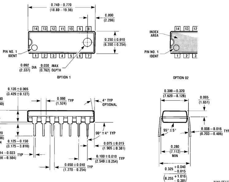
**14-Lead Molded Dual-In-Line Package**
