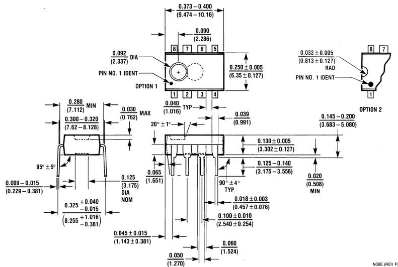
**8-Lead (0.300" Wide) Molded Dual-In-Line Package**
