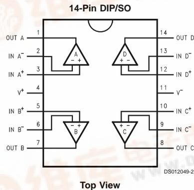
LMC6492 Dual/LMC6494 Quad CMOS Rail-to-Rail Input and Output Operational Amplifier
