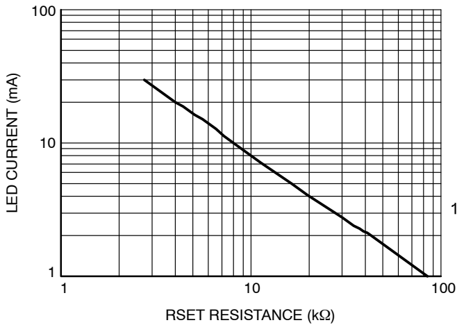
Figure 13. LED Current vs. RSET Resistance
