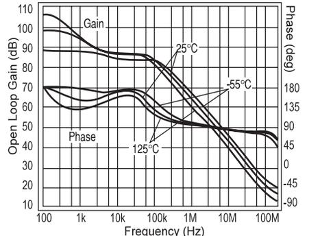
**Non-Inverting Response ( $I_{CC}=5.0\text{mA}$ )**
