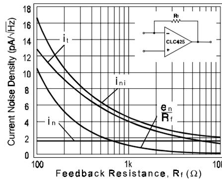
Figure 13: Current Noise Density vs. Feedback Resistance
