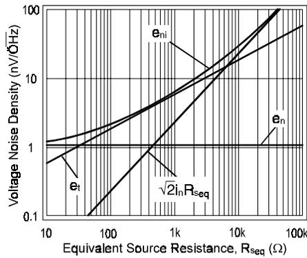
Figure 5: Voltage Noise Density vs. Source Resistance
