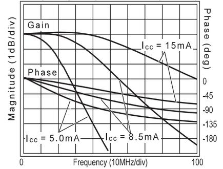
**Open Loop Gain and Phase vs.  $I_{CC}$**
