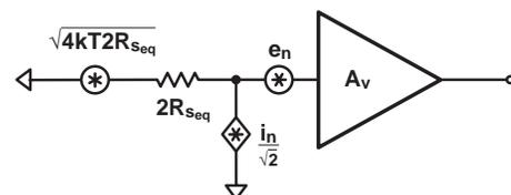
Figure 4: Noise Model with  $R_f || R_g = R_{seq}$
