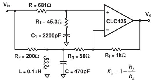
$$\frac{V_o}{V_{in}} = K_o \left( \frac{sC_1 R_1 + 1}{sC_1 (R_1 + R) + 1} - \left( \frac{R_f}{R_f + R_g} \right) \frac{sLR_g}{s^2 LCR_2 R_g + sL(R_2 + R_g) + R_2 R_g} \right)$$
