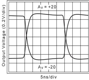
**Large Signal Pulse Response ( $V_o=2V_{pp}$ )**
