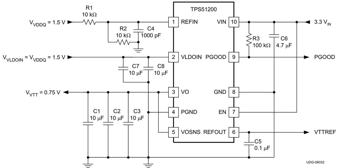
Figure 28. 3.3- $V_{IN}$ , DDR3 Tracking Configuration
