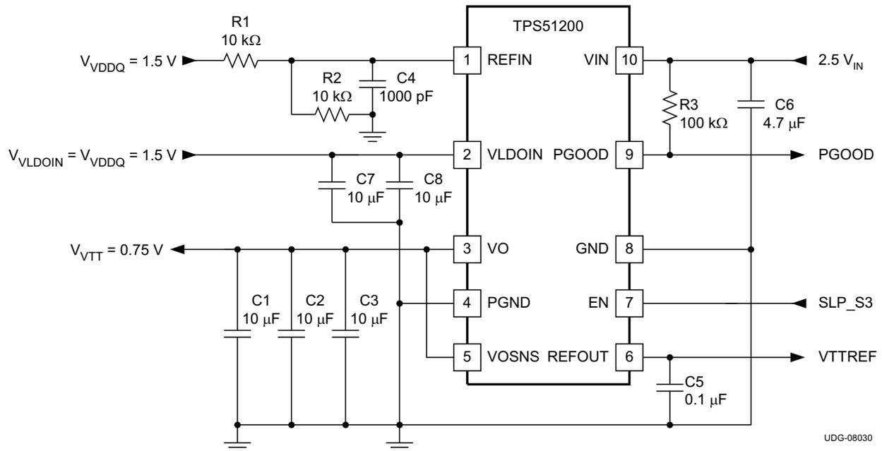
**Figure 26. 2.5-V<sub>IN</sub>, DDR3 Configuration**
