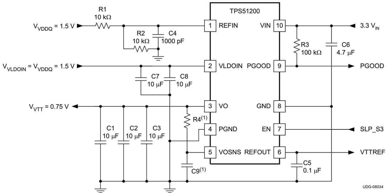
Figure 30. 3.3-V<sub>IN</sub>, DDR3 Configuration with LFP
