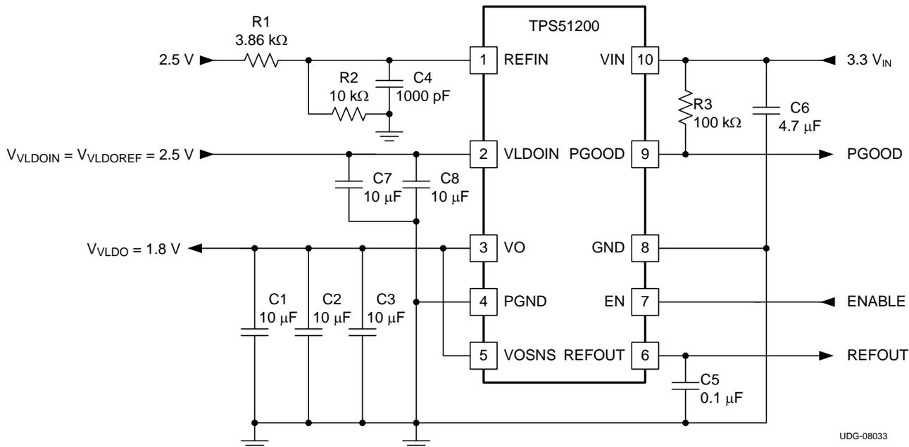
Figure 29. 3.3-V<sub>IN</sub>, LDO Configuration
