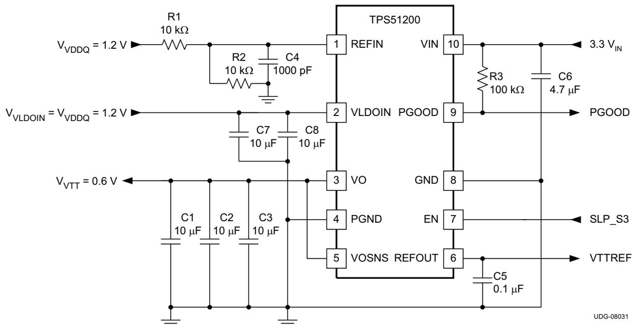
Figure 27. 3.3-V<sub>IN</sub>, LP DDR3 or DDR4 Configuration
