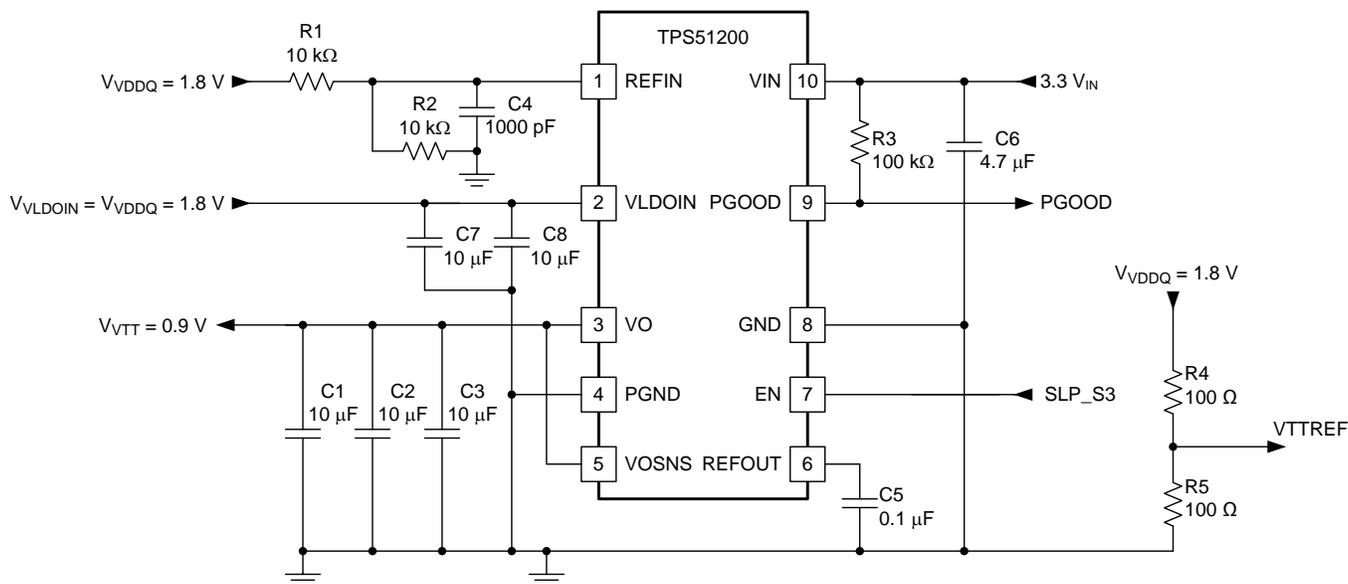
Figure 25. 3.3-V<sub>IN</sub>, DDR2 Configuration
