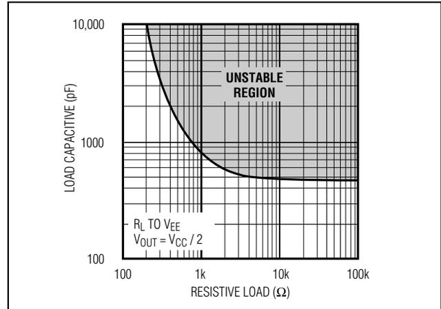
Figure 4. Capacitive-Load Stability
