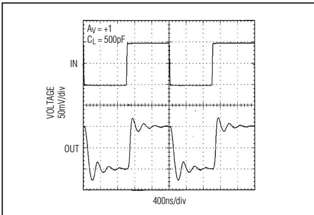
Figure 5. Small-Signal Transient Response with Capacitive Load
