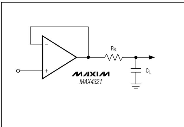
Figure 7. Capacitive-Load-Driving Circuit
