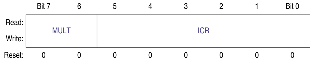
Figure 13-6. IIC Frequency Divider Register (IIC1F)
