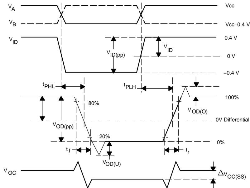
NOTE: All input pulses are supplied by a generator having the following characteristics:  $t_r$  or  $t_f < 100$  ps, 100 MHz from Agilent 81250.  $C_L$  includes instrumentation and fixture capacitance within 0.06 m of the D.U.T. Measurement equipment provides a bandwidth of 20 GHz minimum.
