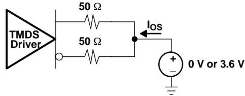
**Figure 3. Short Circuit Output Current Test Circuit**
