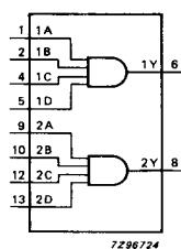
Fig. 4 Functional diagram.
