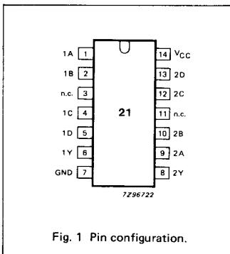
Fig. 1 Pin configuration.
