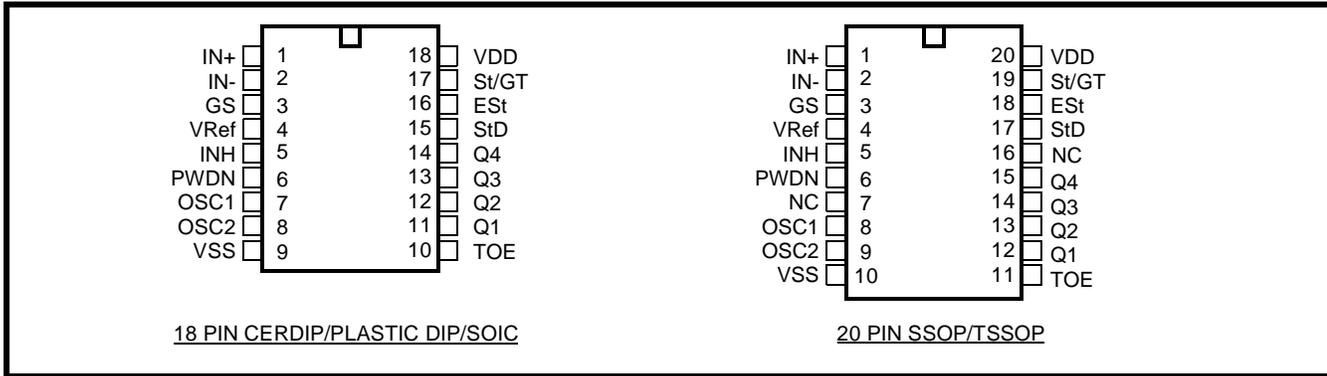
Figure 2 - Pin Connections
