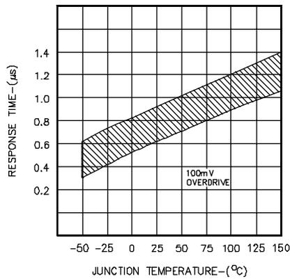
FIGURE 12. COMPARATOR INPUT TO DRIVER OUTPUT DELAY
