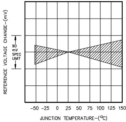
FIGURE 2. REFERENCE TEMPERATURE STABILITY
