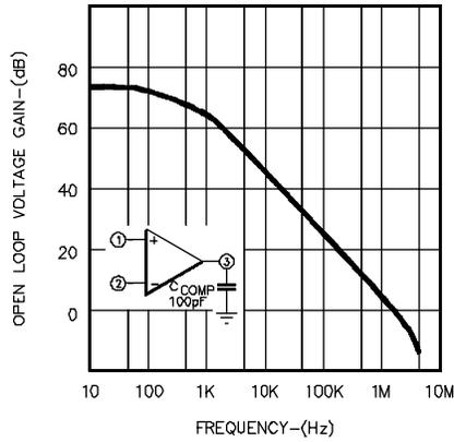
FIGURE 9. ERROR AMPLIFIER OPEN LOOP GAIN VS. FREQUENCY
