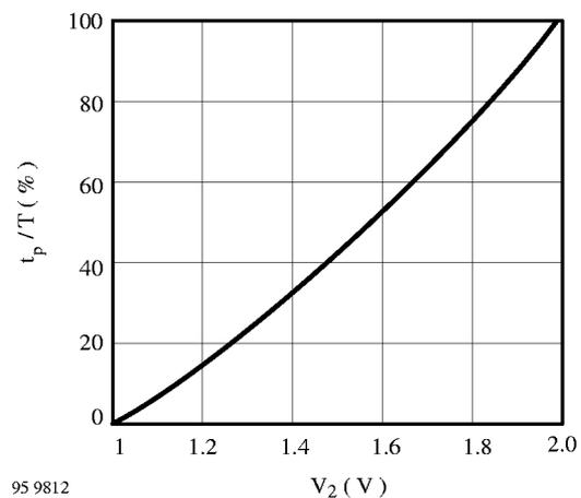
Figure 11. Duty cycle of PWM circuit of figure 9
