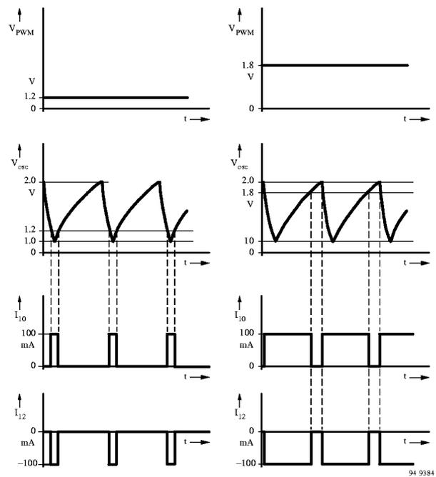
Figure 10. Pulse sequence for PWM circuit of figure 9
