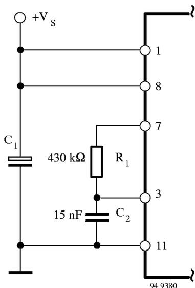
Figure 6. 200-Hz oscillator
