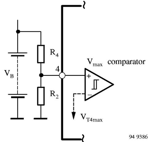
Figure 13. V<sub>max</sub>-comparator circuit
