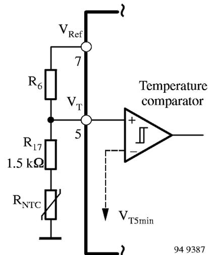
Figure 14. Temperature comparator
