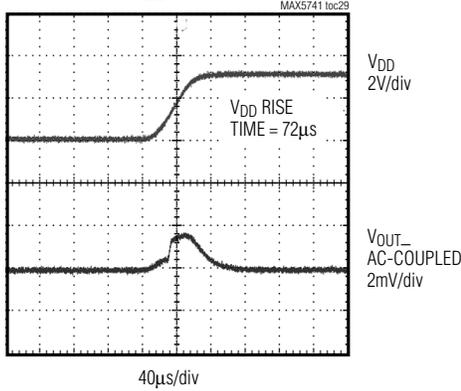
**CLOCK FEEDTHROUGH ( $V_{DD} = +5V$ )**
