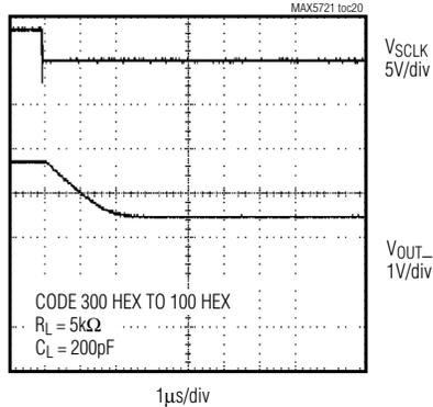
**EXITING POWER-DOWN ( $V_{DD} = +5\text{V}$ )**
