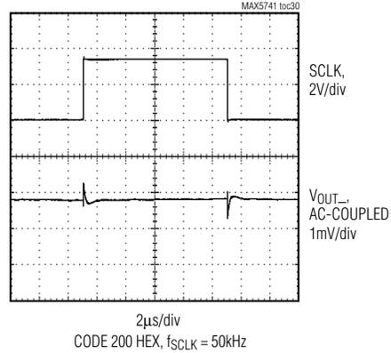
**CLOCK FEEDTHROUGH ( $V_{DD} = +3V$ )**
