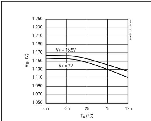
Figure 4. MAX8211/MAX8212 Threshold Trip Voltage vs. Ambient Temperature
