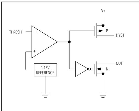
Figure 2. MAX8212 Block Diagram
