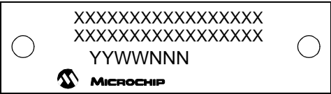
28-Lead PDIP (Skinny DIP)
