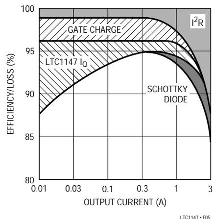
Figure 5. Efficiency Loss
