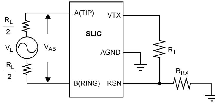
$$I_{L2-4} = 20 \log (V_{TX} / V_{AB})$$
