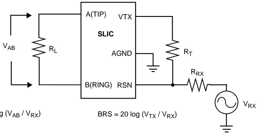
$$I_{L4-2} = 20 \log (V_{AB} / V_{RX})$$
