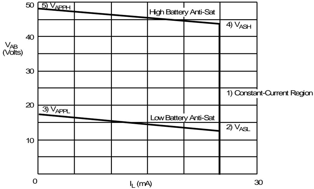
Figure 1. Typical V<sub>AB</sub> vs. I<sub>L</sub> DC Feed Characteristics
