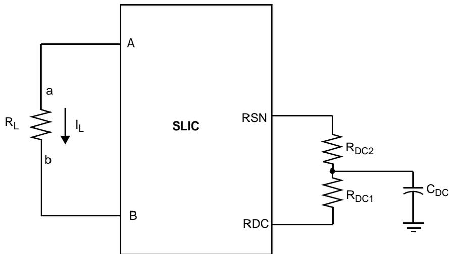
Feed current programmed by  $R_{DC1}$  and  $R_{DC2}$
